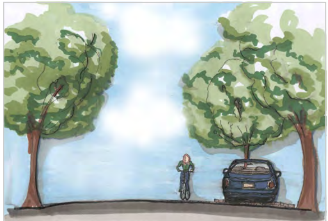
PROPOSED PLAN AND SECTION OF THIRD AVENUE WITH 12 FOOT TRAVEL LANE, AND A COMBINED 5 FOOT BIKE LANE, & 7 FOOT PARKING AREA FOR A TOTAL OF 24 FEET
