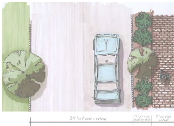
PROPOSED PLAN AND SECTION OF FREMONT AVENUE WITH TWO 12 FOOT TRAVEL LANES AND A COMBINED 5 FOOT LANDSCAPING STRIP AND A 5 FOOT SIDEWALK FOR A TOTAL OF 34 FEET.
